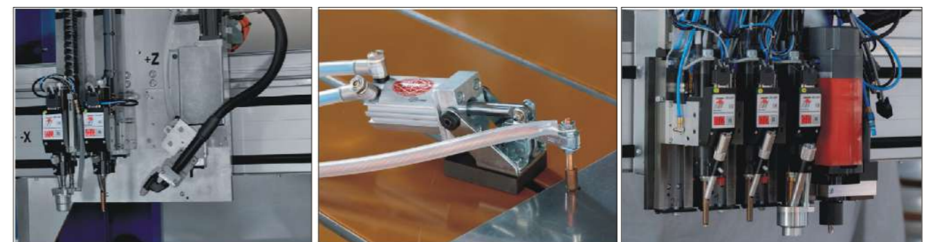
可配置多达四个焊头的焊接设备 Welding equipment for up to four welding heads.
