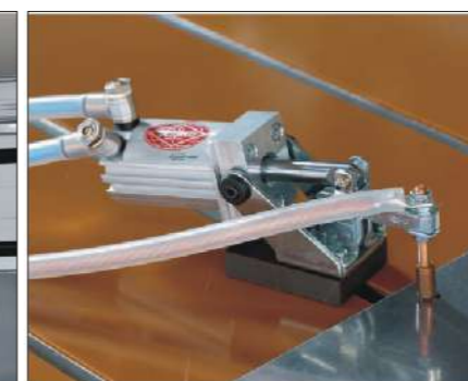
选项: 气动地线夹 Option: Pneumatic power clamp
