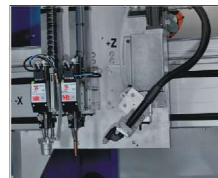
可配置多达四个焊头的焊接设备 Welding equipment for up to four welding heads.
