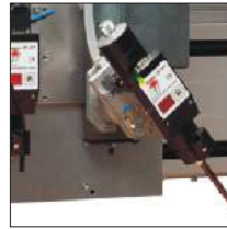
选项：焊头转动轴 Option: Rotatable welding head axis
